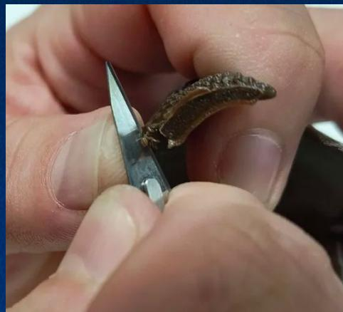
If your slicing profile is not totally accurate, it may cause some overhang due to filament expansion on the support tree mode. You may trim the excesses with a scalpel for better finishing results.
