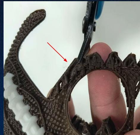
Use a pair of needle-nose pliers to remove the supports. Be very careful not to damage the thinner areas.
