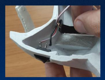
Use double sided tape to glue the battery holder in place inside the Dream Fairy according to the picture.
