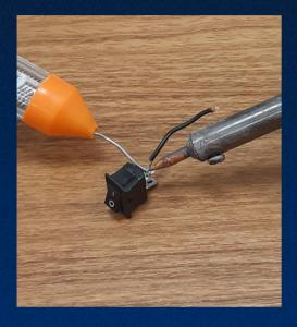
• Thread the red wire through the rectangle hole on the Dream Fairy, then solder its end to the "o" (off) pin on the on-off switch.
