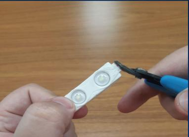
On the end of one module, separate the two wires (the white and the red) from one another. Cut the red wire at a length of 9cm and the white one at a length of 6cm. Strip the ends of both wires in about 1cm.
