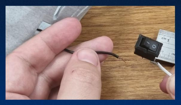
Fit the on-off switch into the rectangle hole made for it on the High Elk, and solder the wire connected to the "o" (off) pin of the on-off switch to the white wire of the LED module.
