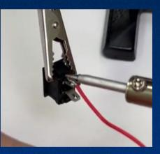
• place the wires through the hole and pass the negative wire through the hole for the DC power jack female.
