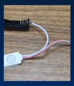
• Cut a separate piece of electric wire of 09cm, strip the ends and solder one of them to the positive side of the battery holder.
