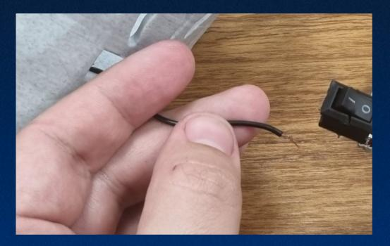
• Fit the on-off switch into the rectangle hole made for it on the Night Owl, and solder the wire connected to the "o" (off) pin of the on-off switch to the white wire of the LED module.
