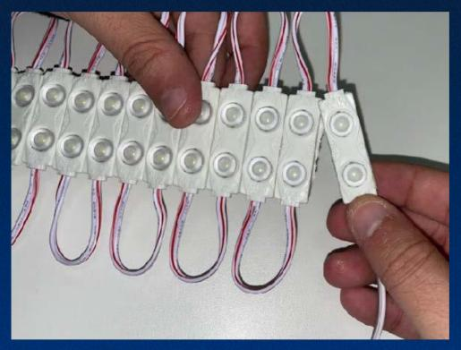
On the end of one module, separate the two wires (the white and the red) from one another. Cut both wires at a length of 9cm. Strip the ends of both wires in about 0,5cm.
