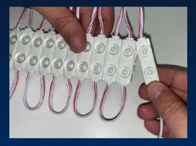
On the end of one module, separate the two wires (the white and the red) from one another. Cut both wires at a length of 9cm. Strip the ends of both wires in about 1cm.
