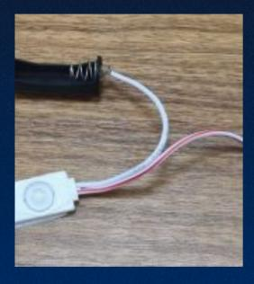
Cut a separate piece of electric wire of 09cm, strip the ends and solder one of them to the positive side of the battery holder
