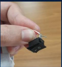
Fit the on-off switch into the rectangle hole made for it on the Pegasus, and solder the wire connected to the "I" (on) pin of the on-off switch to the positive side of the battery holder.
