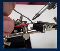
Now pass the negative LED module wire through the DC Plug hole and weld to the DC Power jack female pin.
