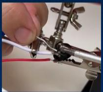
Fit the DC Power Jack female to the printed model
