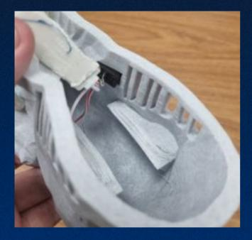
Using their own double sided tape, stick the two LED modules on the inside of the Pegasus on its designated place next to the openings on the model, according to the picture.
